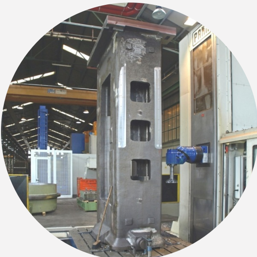
Milling machine PAMA SR1000 with rotating table
